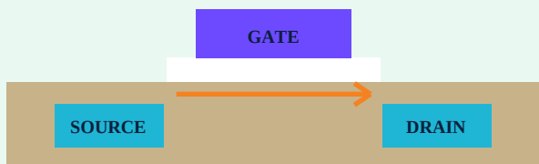
FIGURE 9. An insulated gate controls the channel electrostatically, making MOS technology highly scalable.
