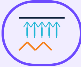
FIGURE 3. The triode's grid controls electron flow, enabling amplification and fast switching without moving contacts.
