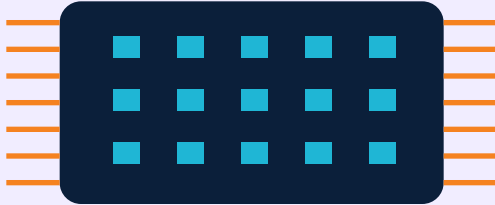
FIGURE 8. Integration replaces hand-wired assemblies with complete circuits created together on a semiconductor substrate.
